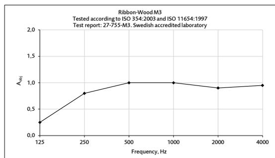
Equivalent absorption area per m<sup>2</sup> screen area (m<sup>2</sup>S / m<sup>2</sup>)
