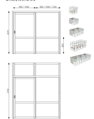
Other dimensions on request. Lowest height 2070 mm. Dividing borders: Standard divisions at 800 and 2070 mm. Thickness: 40 mm Weight: approx. 40 kg / screen
