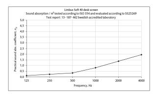
Equivalent absorption area per m<sup>2</sup> screen surface (m<sup>2</sup>S/m<sup>2</sup>)
