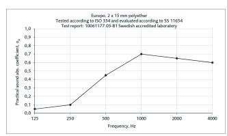
Equivalent absorption area per m<sup>2</sup> screen surface (m<sup>2</sup>S/m<sup>2</sup>)
