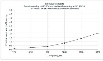
Equivalent absorption area per m<sup>2</sup> screen surface (m<sup>2</sup>S/m<sup>2</sup>) The values are to be multiplied by the screen area.
