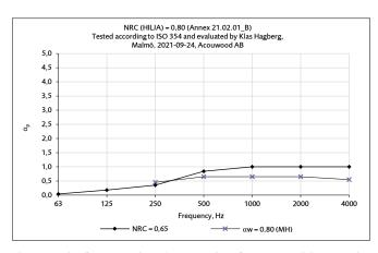
The NRC value for HILJA is based a mean value of one, two and three panels mounted directly to the wall on 7 mm pads and separated by a small distance of 50 mm.
