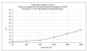
Equivalent absorption area per m<sup>2</sup> screen surface (m<sup>2</sup>S/m<sup>2</sup>)
